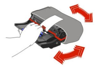
5. Remove all packing materials from the imaging unit.
