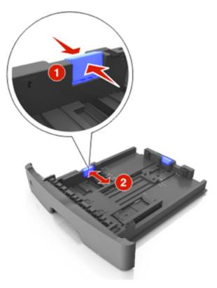
3. Unlock the length guide. Squeeze, and then slide the length guide tab to the correct position for the size of the paper you are loading.
