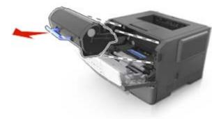
3. Lift the blue handle, and then pull the imaging unit out of the printer.
